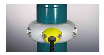
The rope end is pressed into place with a pressed end collar, a 2-part polyamide sphere holds the end of the rope and guarantees a proper seat in the Frox housing. The Frox is connected to the Terranos post using special Terranos clamps made for holding the Frox housing. The dimensional match between the Frox housing and the polyamide sphere allow the connected rope to be aligned in the direction of tension within a specific range. Collars at the sphere prevent damage to the rope at the housing.
