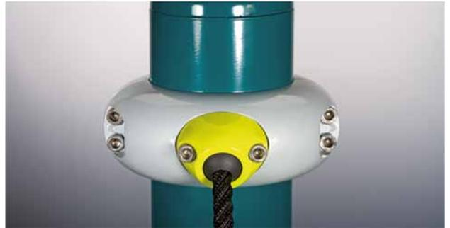
The rope end is pressed into place with a pressed end collar, a 2-part polyamide sphere holds the end of the rope and guarantees a proper seat in the Frox housing. The Frox is connected to the Terranos post using special Terranos clamps made for holding the Frox housing. The dimensional match between the Frox housing and the polyamide sphere allow the connected rope to be aligned in the direction of tension within a specific range. Collars at the sphere prevent damage to the rope at the housing.
