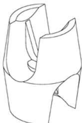
The ball knot before hydraulic pressing
